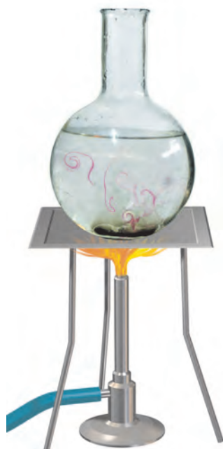
Fig. 4.9 Convection of heat in water
