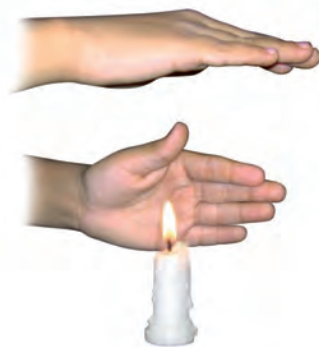
Fig. 4.10 Transfer of heat by convection in air
