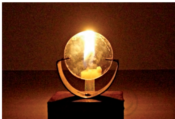
Fig. 15.26 Virtual image formed by the convex lens
