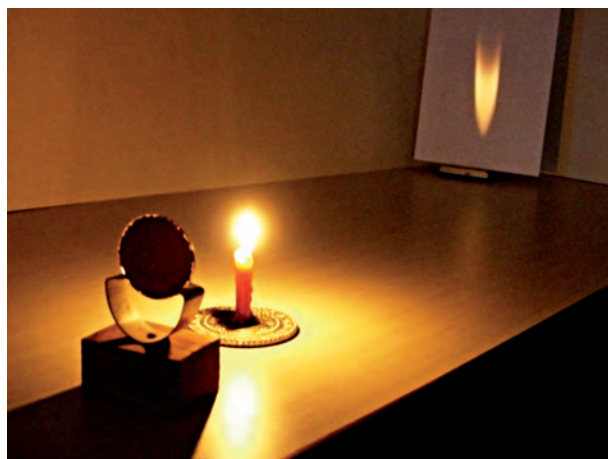
Fig. 15.15 Real images formed by a concave mirror
