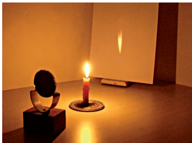
Fig. 15.15 Real images formed by a concave mirror
