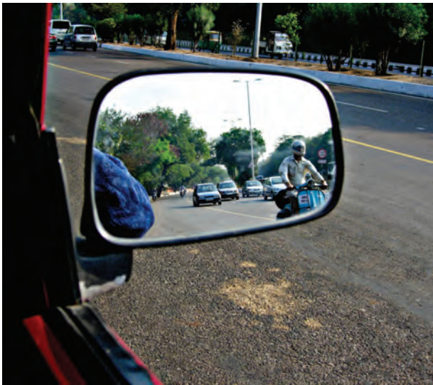
Fig. 15.20 Convex mirror as side view mirror
