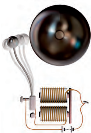
Fig. 14. 20 Circuit of an electric bell
