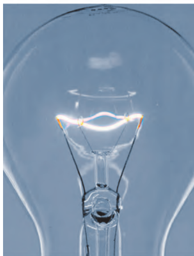
Fig. 14.12 Glowing filament of an electric bulb (incandescent)
