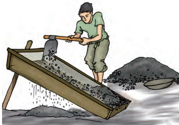
Fig. 5.7 Pebbles and stones are removed from sand by sieving
