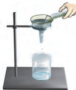
Fig. 5.10 Filtration using a filter paper
